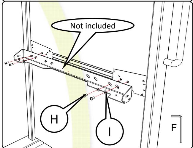
**6** Mount the BalanceBox®650 on the wall bracket and assemble the screws at the top (● 5 mm)
