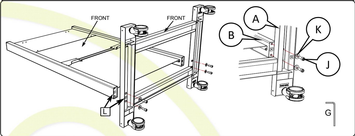
**4** Assemble the handle to the frame (● 5 mm)
