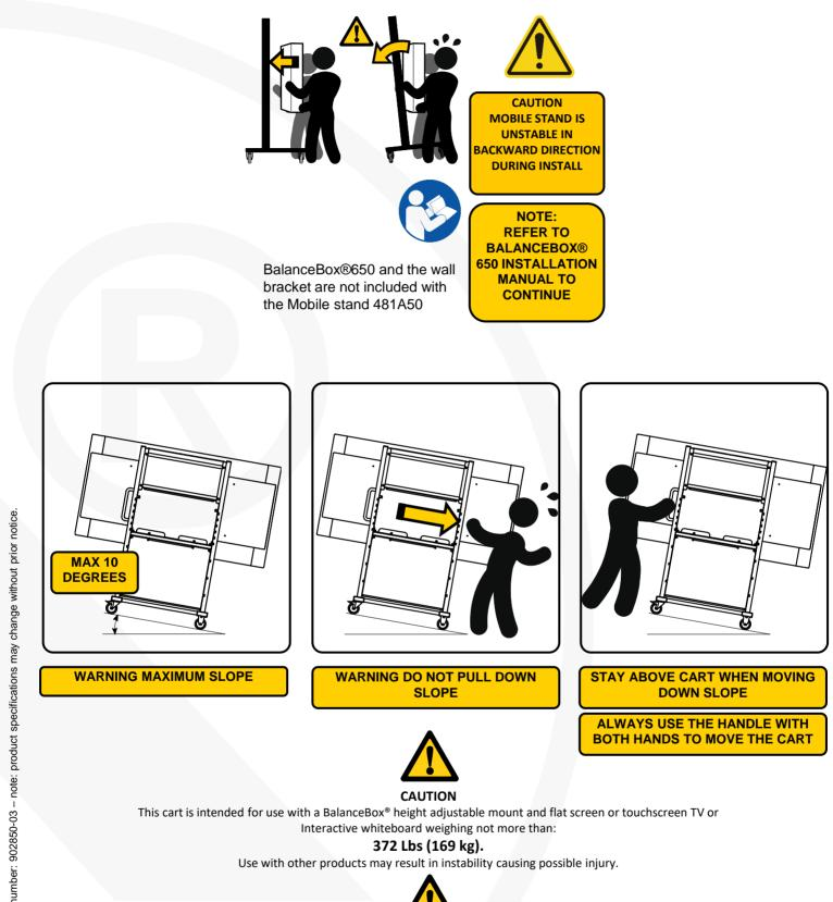
CAUTION "This cart is Intended for use only with the maximum weights indicated. Use with products heavier than the maximum weights indicated may result in instability causing possible injury."
