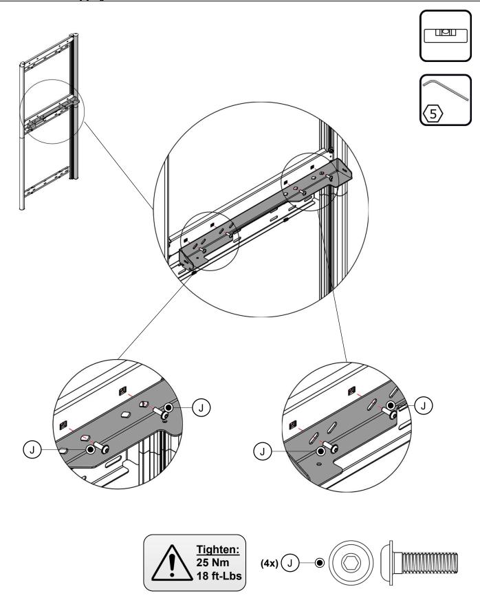
Use 4 screws [J] to secure the BalanceBox® 650 at the top.
