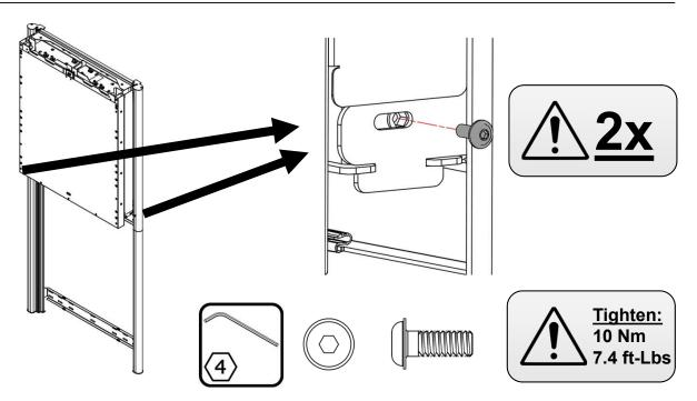
**13** After mounting the BalanceBox® 650, place all covers back according to the manual.
