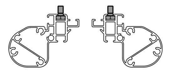
Place all 3 wall brackets [C] over the screws and mount each wall bracket with 4 nuts [L] Make sure the middle wall bracket connects the aluminum profiles.
