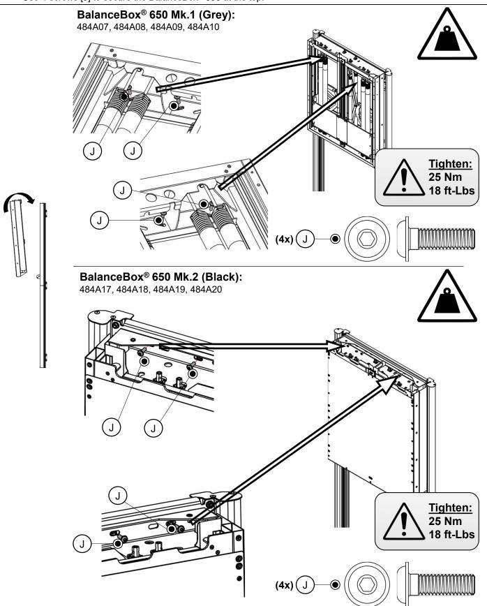
**12** Secure the BalanceBox® 650 on each side to the wall bracket. Use 2x screw included with the BalanceBox® 650.
